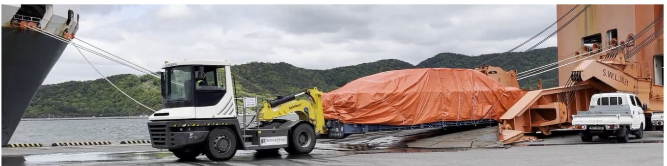
Ro-Ro shipping using a Mafi trailer
